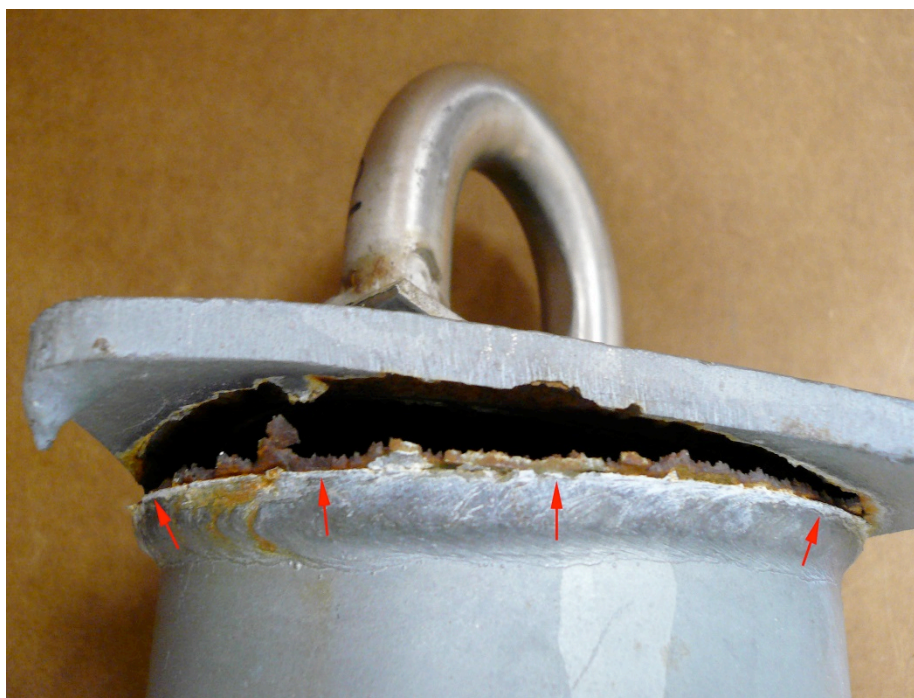
As-received for analysis. Figure 4. Reduced size. Roof anchor #2. Red arrows point to the fractured region.
