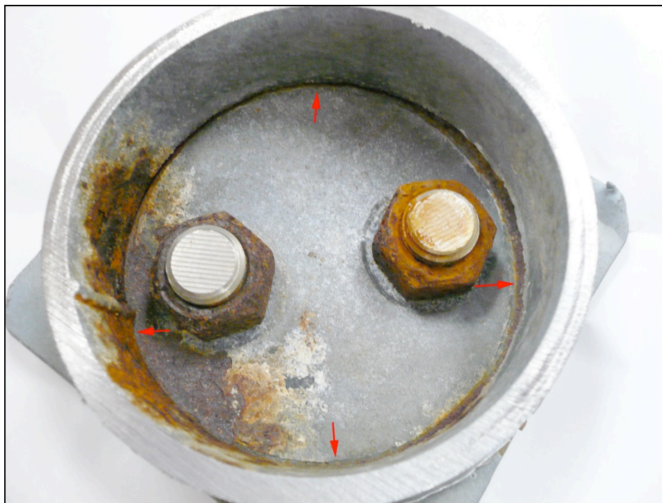
As-received for analysis. Figure 5. Reduced size. Roof anchor #2. Micro-image illustrates inner condition of the roof anchor.
