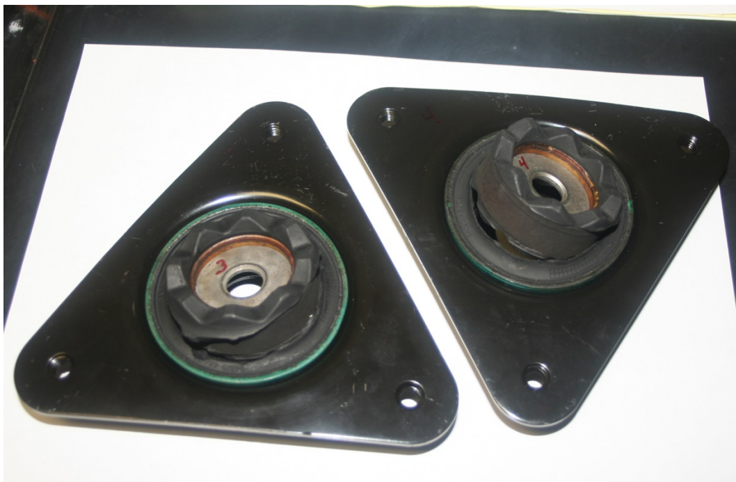
Samples 3 and 4 – Rubber to plastic bond failure samples
