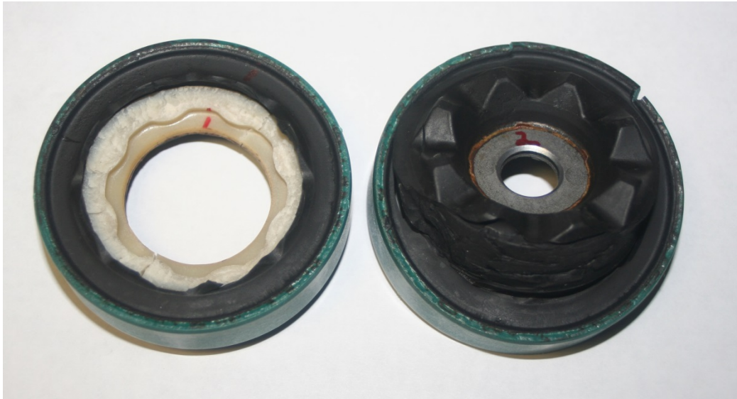
Figure 1 – Samples 1 and 2 No rubber to plastic failure
