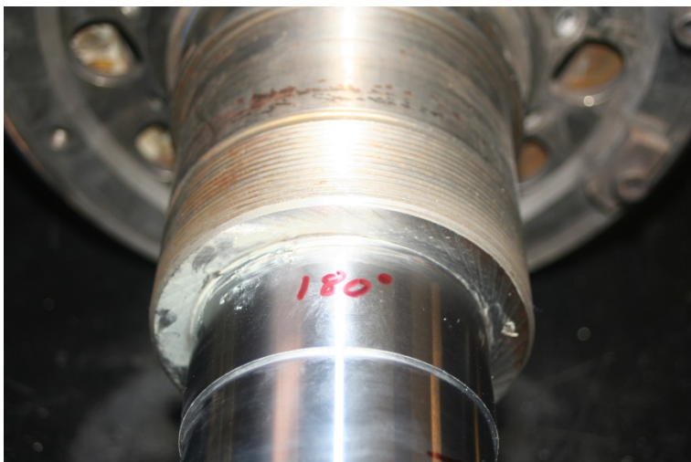
Figure 4 – 180 deg crack propagation
